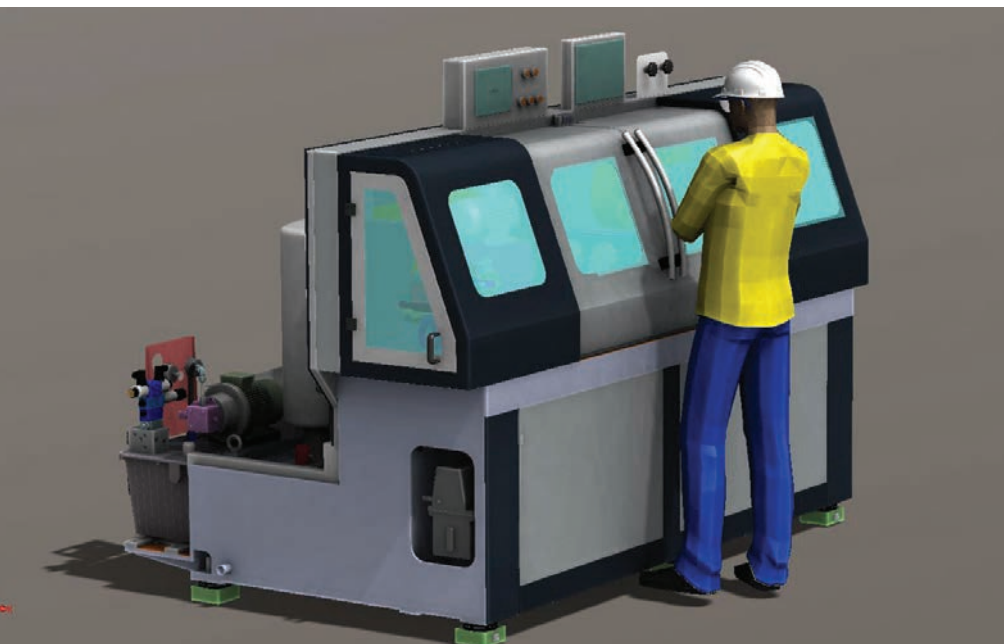
Gun drilling machine design using SolidWorks software
